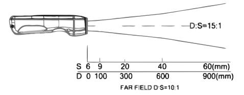
Emissivity: Adjustable 0.10 - 1.00 (EM opt.) Preset 0,95 Digital interface: USB (EM opt. cable and software)
