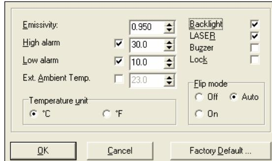
A reset of the unit to the factory default values [**► Reset**] will delete the display of this function during operation [**Setup Menu 2**].
